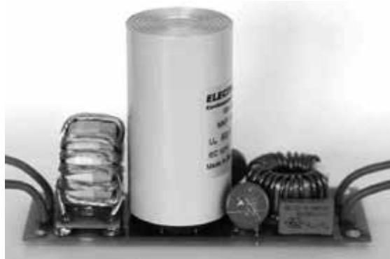
The „LCDC“ (DC buffer circuit with low, or small, capacitance) complies with all these requirements and has become possible with the high density DC film capacitors designed and manufactured by ELECTRONICON.
