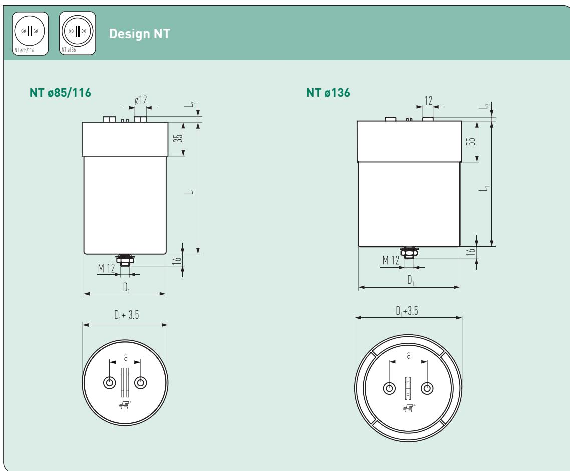
**E50 CAPACITORS WITH A CAN DIAMETER OF 85...136 mm**
