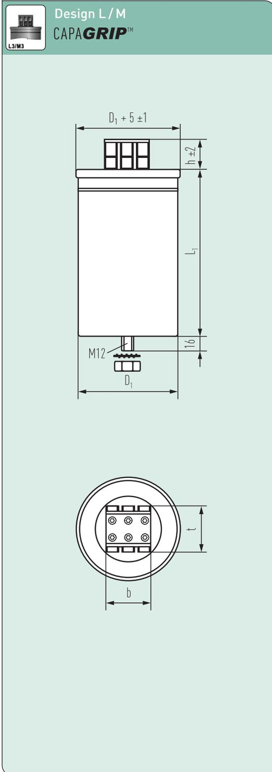
**CAPACITORS WITH A CAN DIAMETER OF 75...136 mm**
