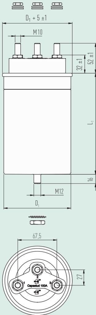
**CAPACITORS WITH A CAN DIAMETER OF 116/136 mm**
